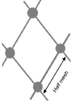
**Half mesh:** the distance from the center of one knot to the center of the next knot in the square mesh.
